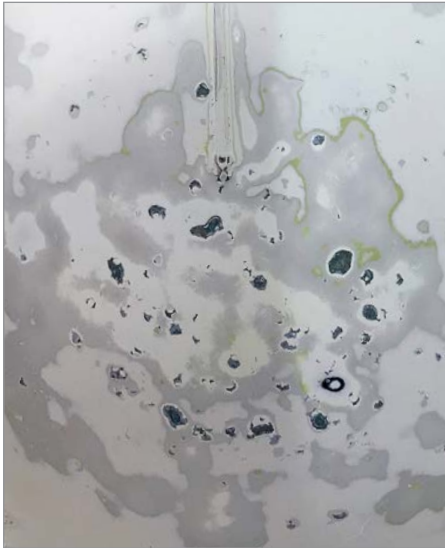
Close up view of damaged radome flow without protective boot installed.
