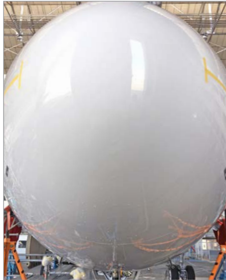
Protective boot installation on radome with internal static diverters.
